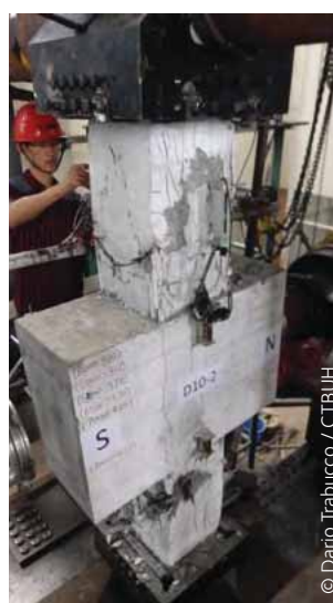
Figure 3.11: Scaled (1:6) Specimen tested to failure
