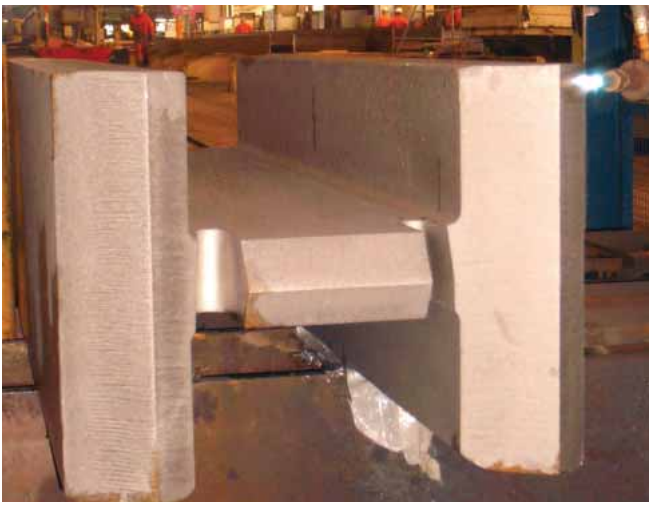
Figure 6.12: Bevel preparation on Jumbo
