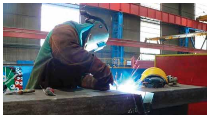
Figure 2.5: Welding of HISTAR® structural steel grades without preheating* (CJP_Complete Joint Penetration_splice of HD400 x 1299 in HISTAR® 460)
