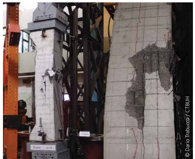
Figure 3.9 Mega-Column scaled (1:4) Specimen tested to failure
