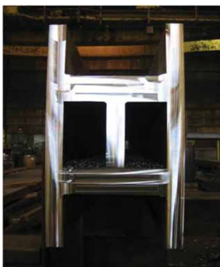
Figure 3.5: Rolled section with coverplates
