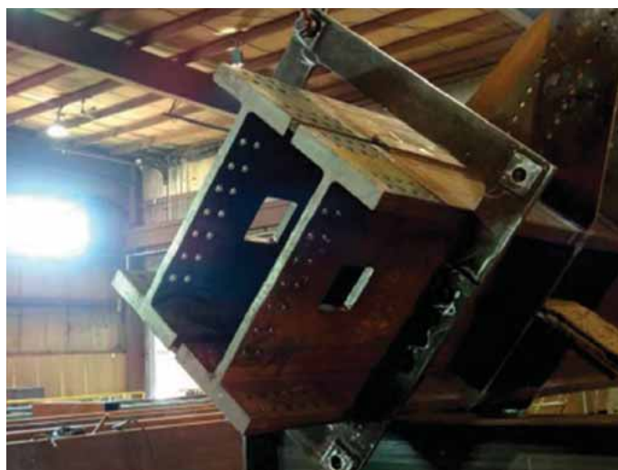
Figure 3.6: Welded sections, Two heavy sections welded together
