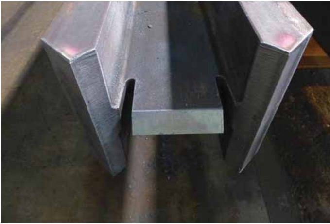
Figure 6.3: CJP butt weld preparation for Jumbo column
