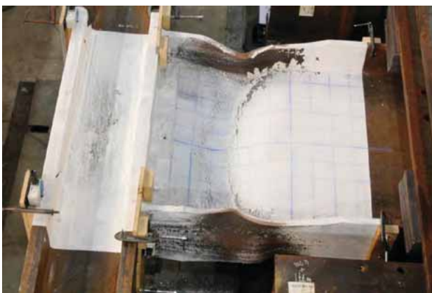
Figure 10.6: RBS: Reduced Beam Section Plasticisation
