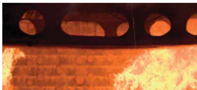
Figure 8.5: Fire test on unprotected cellular beams (Fracof)
