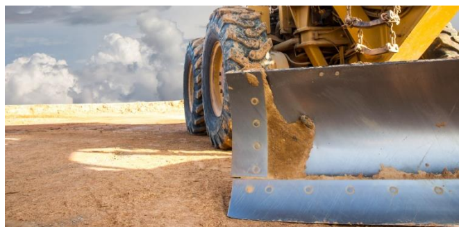
Relia®: Up to six times better abrasion properties than normal steel © Shutterstock/yuttana jeenamool
